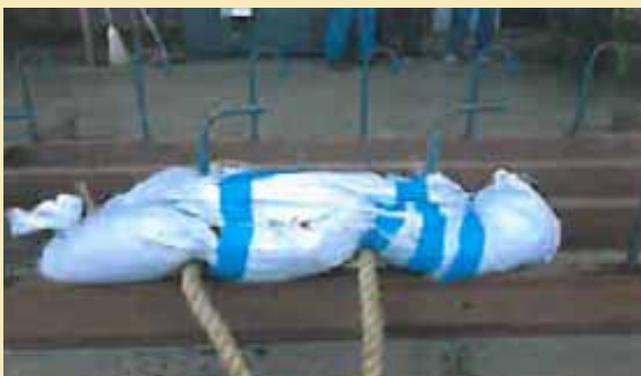
The photograph on the left clearly illustrates that “rebar dowels fabricated with 90 degree bends and caned ends” DO NOT provide any protection from impalement.
